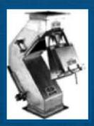
Hump magnet separators are used to remove ferrous contaminants iron nuts, bolts, wire etc. from the conveyed material. With the hinged doors, cleaning the magnetic surface is quick and easy. The unit can be mounted directly in the air stream with the square to round transitions, which can be provided. Hump magnetic separators consists of two plate magnets, which are hinged and gasketed to the rugged steel housing. These plate magnets can be unlatched and swing open for quick manual cleaning.
