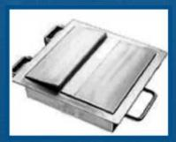
Plate magnets are important industrial separators that are meant for the separation of fine ferrous materials and large pieces of tramp iron, from many types of free flowing and pneumatically conveyed material such as corn, sugar, flour, gravel& plastic etc. The plate magnets also goes very well with powdery, moist, lumpy, and abrasive products and large debris that might choke, bridge, or cause rapid wear in cartridge-based
