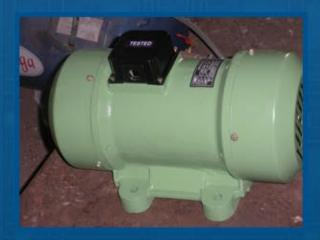
The vibratory motors preffered by us are fully enclosed with 3-phase squirrel cage induction motor that has adjustable eccentric weight mounted on both the end of shaft. By adjusting both eccentric weights, we can easily vary the rate of vibration. The selection of shaft material and bearing should be carefully done to withstand heavy radial load.
