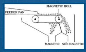
A short special fabric conveyor belt covers the magnetic roll and a tensioning idle roll driven by a motor. A feeder discharges material on the belt on continues controlled rate of flow at uniform layer thickness. The ferromagnetic and paramagnetic particles adhere to the belt while the non-magnetic particles flow freely off the end of the conveyor. The division of paramagnetic and non-magnetic
