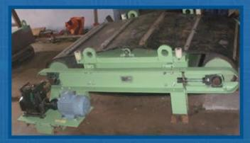
Our wide array of manufactured magnetic equipments comprises of suspended magnets and over band magnetic separators. For automatic and continuous separation of tramp iron from the product, our powerful over band self cleaning electro-magnetic separators are used to remove the tramp iron flowing along with the product on a belt
