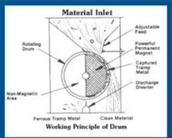
The permanent Magnetic Drum consists of stationery permanent Magnetic assembly having uniform and everlasting Magnetic field across the entire width of the drum, which is effective over approximately half the drum circumferences as shown in fig. Drum shell made of non-magnetic stainless steel revolves around the magnetic field.
