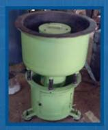
Vibro finishing machine is a bowl type centrifugal finishing machine. The machine bowl is loaded with suitable ceramic / plastic or steel media and the components to be processed. The mutual rubbing action takes place inside the chamber due to the gyratory vibrations, Compared to other simpler processes this method completes the deburring process faster.
