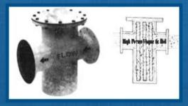
The liquid line separators developed by us are designed for heavy-duty large volume liquid and semi-liquid line flow system. This employs a slip in cage of stainless steel permanent magnet tubes, which is used to capture tramp metal particles, migrate to the rear of tubes, where they remain safe from wash off unless these are not cleaned. These tubes are hanged on top access bolt on steel plate and seal, which is easy to clean. The magnet cage
